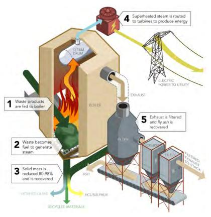
steam, which is usually converted to electrical power and sold to an electrical utility.
